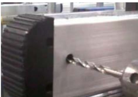
1.Unbolt and remove old foot. Put a new foot in and Drill a M6 through the hole and foot.
